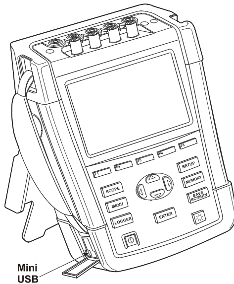
Figure 25-1. Location of USB interface connector
